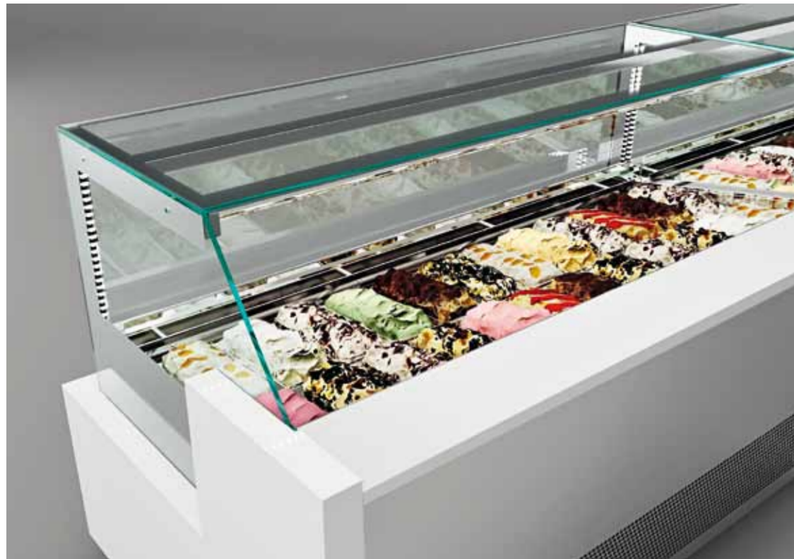
Piano mescola e top operativo. Piano mescola in vetro 10mm serigrafato (RAL 9006). Top operativo in composto acrilico 100% riscaldato, spessore 13mm. Top glass and worktop. Silk-screen print top glass 10mm thick. Heated worktop, acrylic solid surface finishing, thickness 13 mm.
